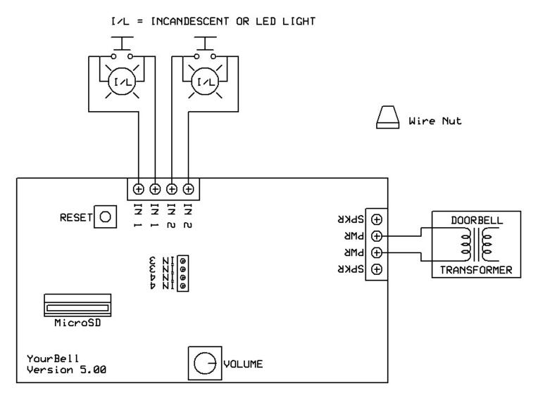
This is the preferred wiring for the YourBell Version 5.00. The location of the wire nut is found and the 3 wires disconnected. The original 6 wires are now connected to the YourBell.
