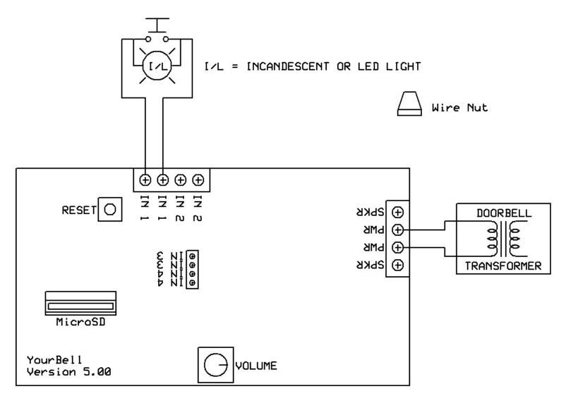
This is the preferred wiring for the YourBell Version 5.00. The location of the wire nut is found and the 2 wires disconnected. The original 4 wires are now connected to the YourBell.
