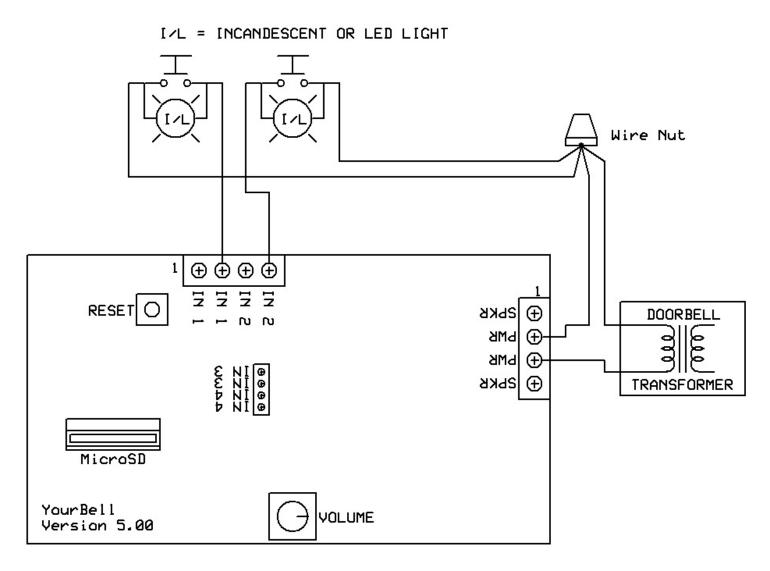
This is the 4 Wire method of wiring the YourBell Version 5.00. The buttons and the YourBell are connected to the transformer using the wire nut. The locations of the wires on the two terminal blocks is important.
