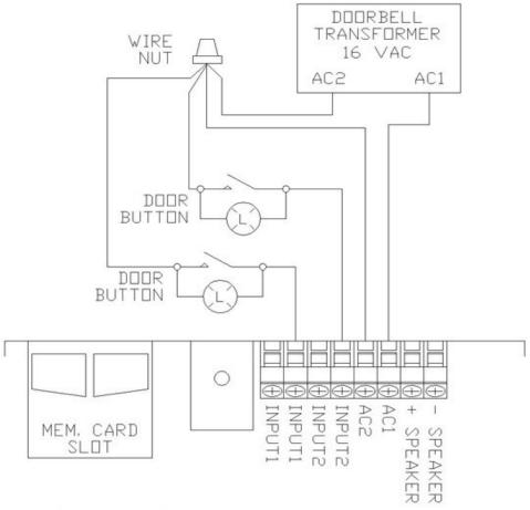
This is the 4 wire method of wiring the YourBell. The wire for AC2 will be connected to the transformer, and the door button via the wire nut.
