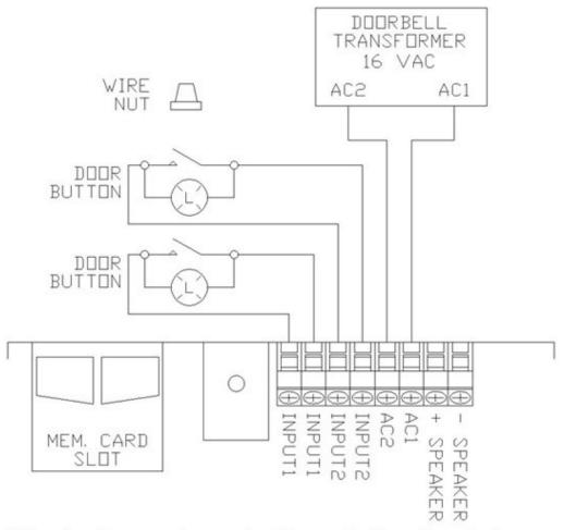
This is the preferred wiring of the YourBell. The location of the wire nut is found and the 3 wires disconnected.
