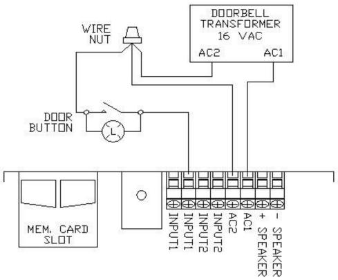
This is the 3 wire method of wiring the YourBell. The wire for AC2 will be connected to the transformer, and the door button via the wire nut.
