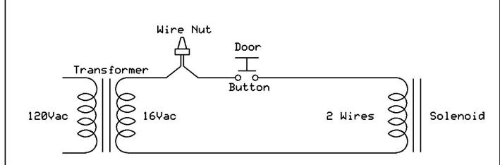
This is how the electrician ended with 2 wires.
