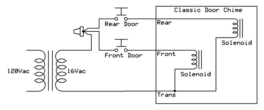
This is how the electrcian ended up with 3 wires coming out of the wall. Each door button is wired to be an on/off switch. Each press of a door button energizes a solenoid, a plunger is extended hitting a metal plate and a noise is made.
