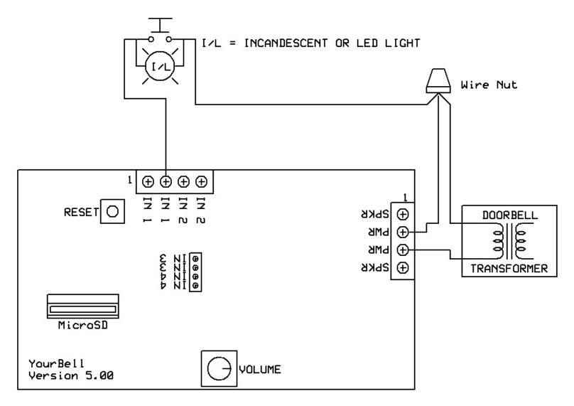
This is the 3 Wire method of wiring the YourBell Version 5.00. The button and the YourBell are connected to the transformer using the wire nut. The locations of the wires on the two terminal blocks is important.
