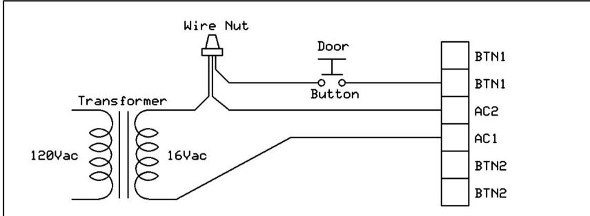
This is the 3 wire metod of wiring of the Yourbell. The wire for AC2 can be connected to the transformer, the wire nut or the door button.
